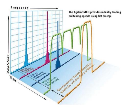
FIGURE 1: MXG switching speed.
